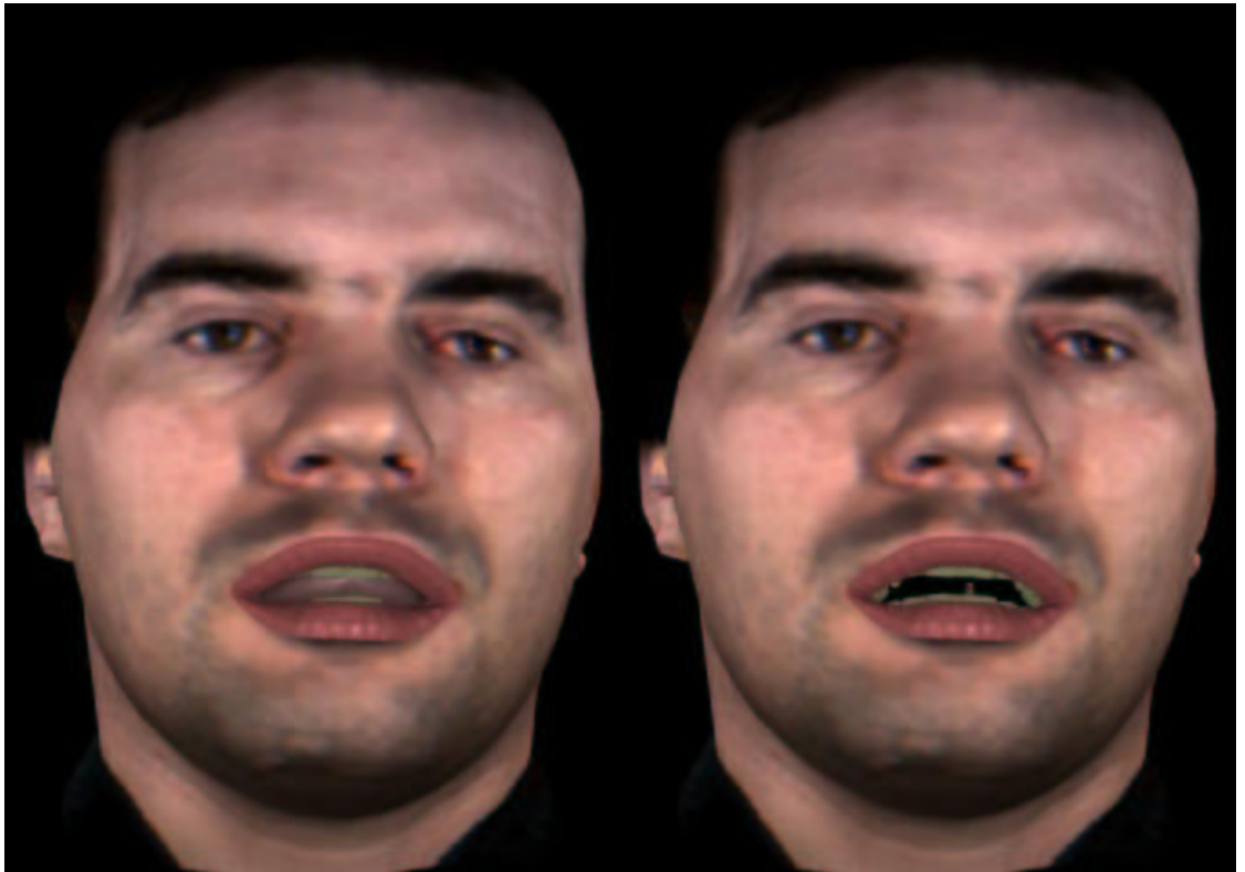
Figure 4.6: A side-by-side comparison of our facial model in the phoneme position /n/. On the left our tongue model has been added to the facial model, while on the right there is no tongue. The visible artifacts in the mouth on the right side are the back sides of the triangles from the rear of the head.
