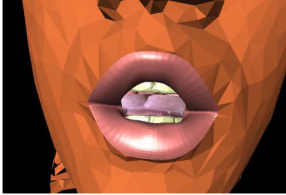
Figure 3.5: The lip model grafted onto face geometry. This is from our real-time TTAVS system using OpenInventor to render the frames.
